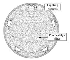
Fig. 4 The lighting fixtures fixed in base
