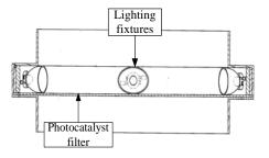
Fig. 5 The front view of photocatalyst filter in base
