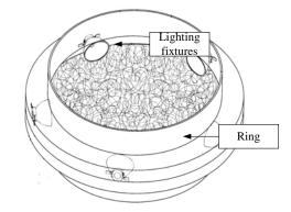
Fig. 3 The photocatalyst filter fixed in base
