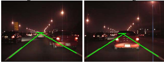
Fig. 9 Results of lane detection when cars moved on the road.
