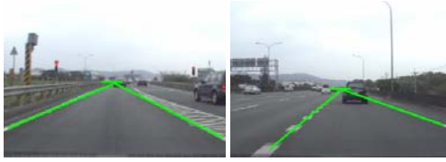
Fig. 6 Detection result of lanes with different types.
