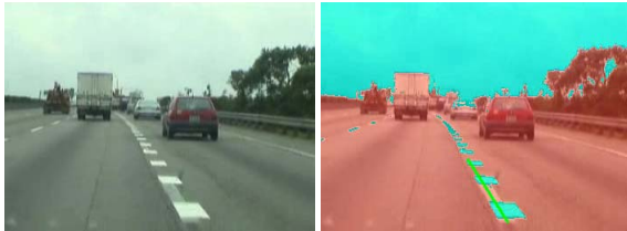
Fig. 10 Lane departure detection.
