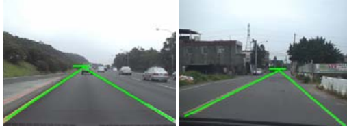
Fig. 7 Detection result of lanes with different colors.
