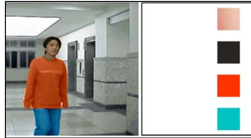
Fig. 6 The pseudo-colorizing and palette mapping
