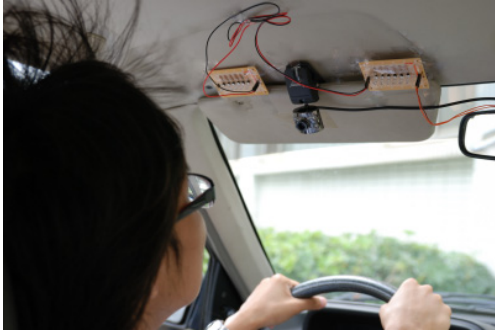
Fig. 11. The illustrations of our experimental vehicle mounted the two-side IR illuminator.
