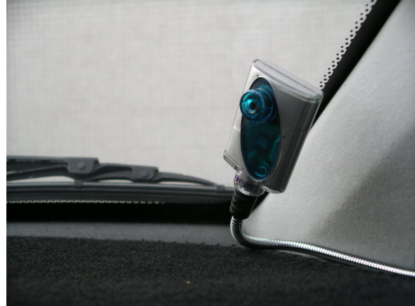
Fig. 14 The USB CCD mounted behind the right front windshield
